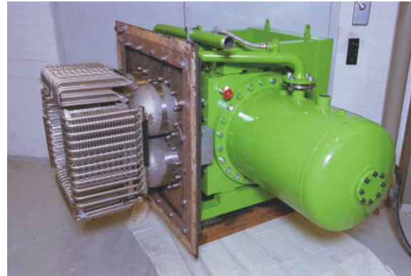
Figure 7. 35 kW Stirling engine before installation in the furnace
